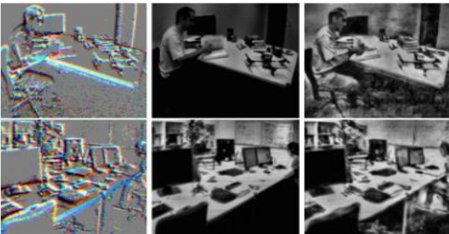
Figure 3. From left to right, input events, active pixel sensor (APS) images from the DAVIS camera, and our results. Our methods construct HDR images with more details that normal cameras could not reproduce as in APS frames.
